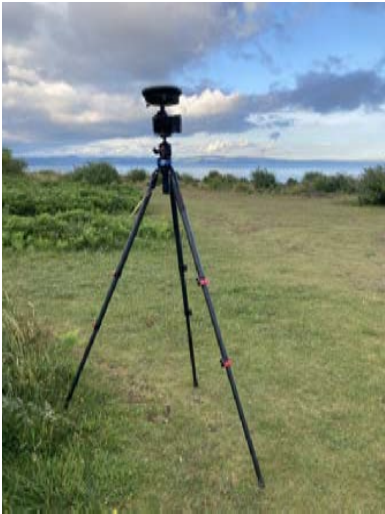
Manfrotto tripod with GS16 antennae
