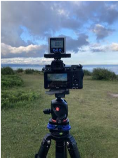
Three-way levelling base and inclinometer
