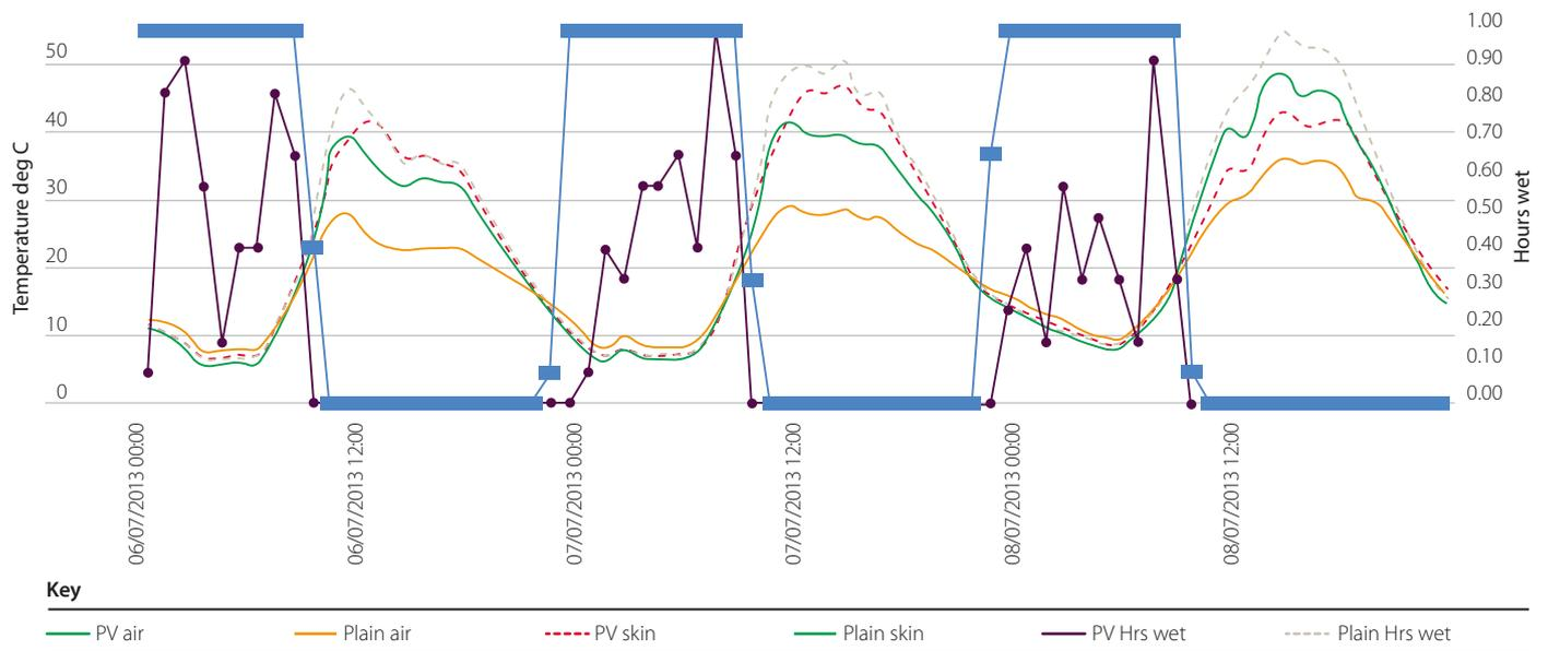
These factors combine to create a significantly more aggressive local corrosion environment underneath the PV panels.
